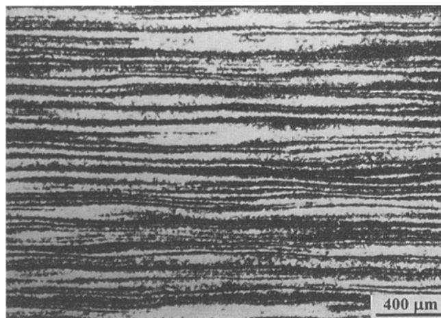
Fig. 2 Dark and white contrast produced after etching
