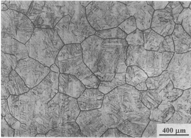
Fig. 7 Microstructure of the specimen after homogenization treatment
